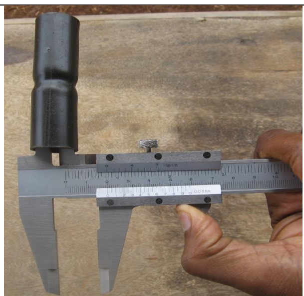
Figure 2.2: Measuring inside diameters of uPVC repair coupling with vernier caliper
