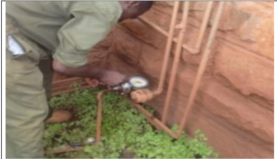
Figure 6.3: Pressure gauge installed at customer metering point
