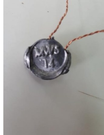
Figure 8.10: Sealing lead stamped by Pliers No. MWS14
