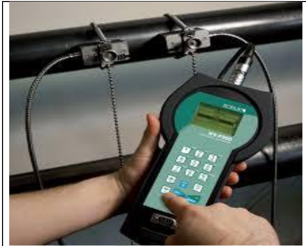
Figure 5.15: Side-mounted sensors on PVC pipe
