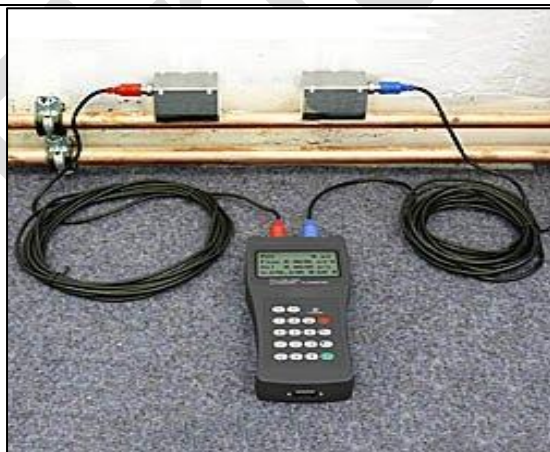
Figure 5.9: UFM mounted on pipe
