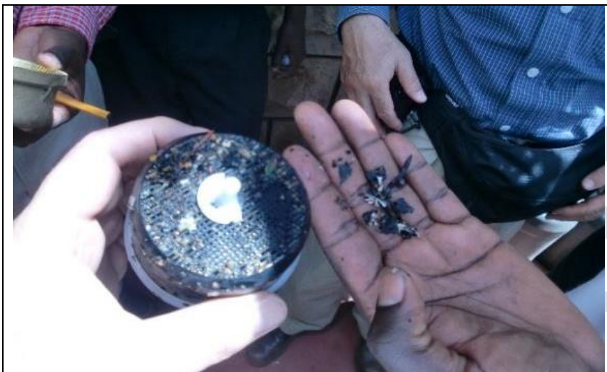
Figure 8.3: Debris trapped meter strainer
