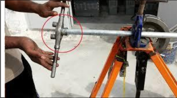
Figure 2.31: Threading of pie with diestock
