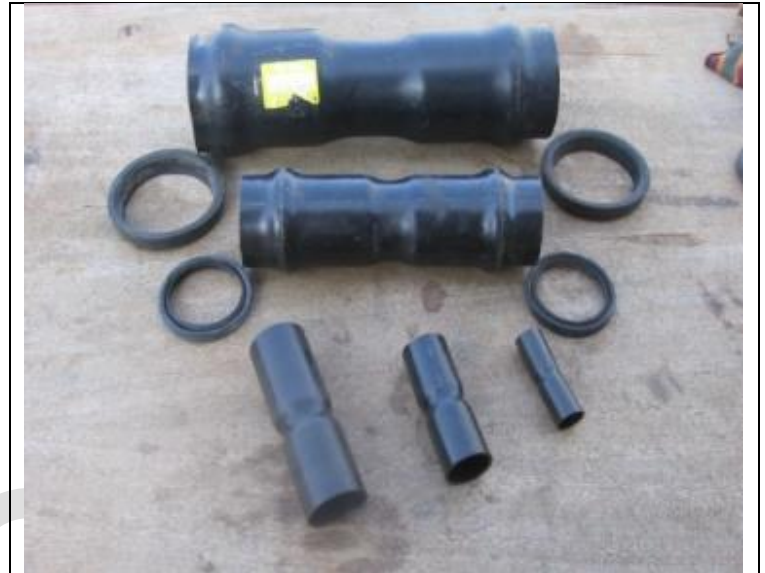
Figure 2.4: Rubber ring couplings (dia \geq 63\text{mm} ) and Bonding Joint Couplings (dia < 63\text{mm} )
