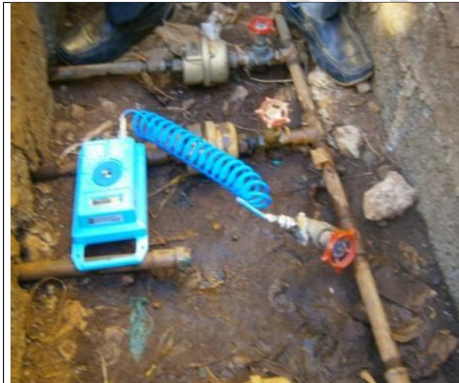
Figure 6.6: Pressure Logger Installed on Pipe
