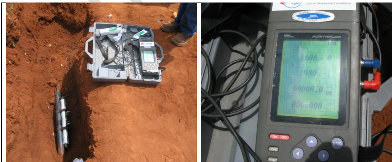
Figure 5.30: Flow Measurement Using UFM
