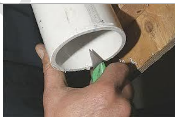
Figure 2.7: Unchamfered dimensions being deburred
